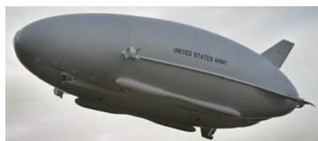
The US Army hybrid airship (LEMV pictured left –  $38,000 \text{ m}^3$ ,  $1.34 \times 10^6 \text{ ft}^3$ ) subsequently was designed, built, inflated/assembled at Lakehurst, flown once (8 Aug 2012) and then mothballed.
