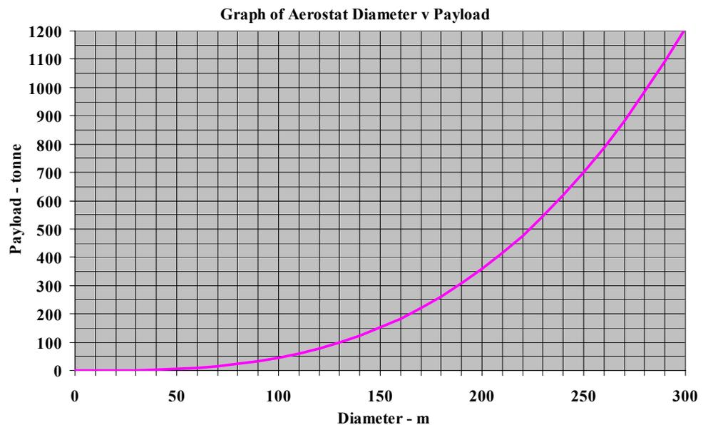
an AeroRaft version with diameter of its length thus would be within range of the upper 1000 tonne goal, so is a viable future objective worth pursuing. It appears to be one of the only viable aerial ways that doesn't need a place to land for payload delivery or extraction!
