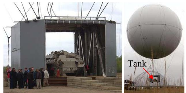
It would have been easy to scale the AirCrane up for much bigger/heavier payloads because the physical relationships work favourably, where aerostatic lift capacity (buoyancy) is proportional to volume and volume is proportional to diameter cubed. Also, balloon weight is proportional to surface area, which is proportional to diameter squared. So basically, balloons get more efficient as size increases and a little bit bigger enables a lot more lift capability!
