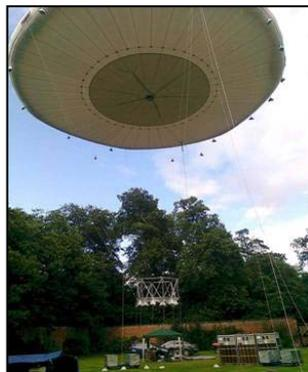
designed to carry a 200 kg load. Vikki was successfully trialled in 2010, proving that the arrangements can be managed using its restraint system, which has been operated safely up to 35 m above the ground.
