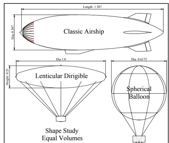
The main benefit of a spherical balloon with a hanging basket is its simplicity (little to go wrong), where the low suspended weight keeps it upright and it doesn't need to face any particular direction. The AeroRaft thus was arranged in a similar way; not needing fins to stabilise pitch and roll aspects, where it remains upright as a pendulum. It then only needed power and propeller systems to be added.
